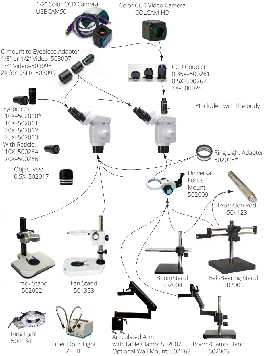
Fig. 3—This diagram shows many of the options available for the PZMIV.
