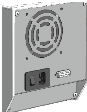
Fig. 6—The back panel has the power switch and plug.
