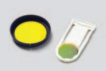
Fluorescence filter sets for ringlights This filter set consists of an excitation filter installed in the light source, and a cut-off filter installed in the light path of the lens. The set is employed to examine fluorescence in the visible range.
