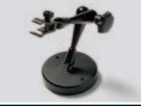
Adjustable stand for flexible lightguides Consists of a heavy base plate and an articulated arm that can be swivelled in all directions. It is attached by only one locking screw and is fitted with a universal and protective light guide holder. Alternatively, the articulated arm can also be attached by means of an M6 thread or an M8 adapter, without the base plate.
