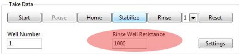
Fig. 35 — When you press the Stabilize button, the resistance of the test resistor displays briefly.
