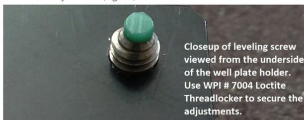
Fig. 50 — The leveling screw, secured with Loctite, is shown from the underside of the well plate holder.
