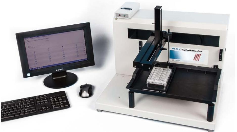
*Fig. 1 — The REMS AutoSampler includes the computer with all the hardware and software installed, the REMS Interface Unit, the robotic arm, a dummy electrode and one measurement electrode.*
