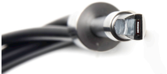
On this dual excitation probe, the LEDs in the center of the probe are illuminated, while the exterior ring of LEDs is dark.
