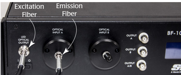
Fig. 11—Press the SMA connectors into place and tighten the nut to ensure that stray light does not enter the fiber connection.
