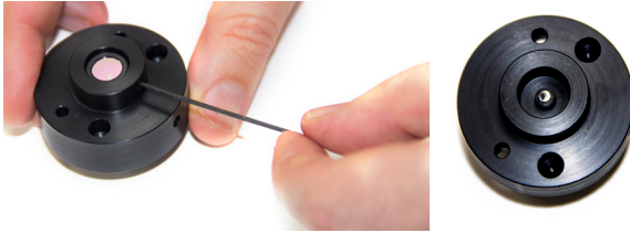
Fig. 15—(Left) Use the specific filter key tool to loosen the filter set screw.
