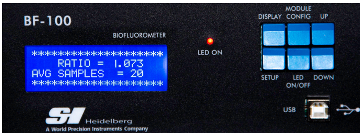
Fig. 4—The display (left side) shows the actual ratio measurement. The six control buttons (right side) let you setup the configuration parameters, turn the LEDs off and on, and manipulate the display.
