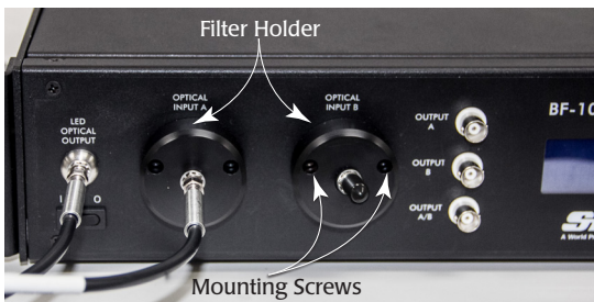
Fig. 12—The filters are located inside the filter holders.
