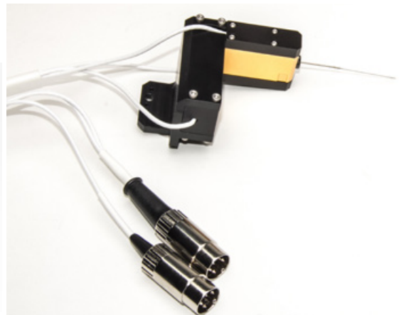
Fig. 6—(Left) The force transducer (sensor assembly) is packaged in a sturdy box to protect the sensitive assembly, and it should always be stored in the case to protect the delicate tip. Fig. 7—(Right) The force transducer has a colored band on one cable to indicate which connector plugs into the Transducer Tweezer port on the Position Control module.
