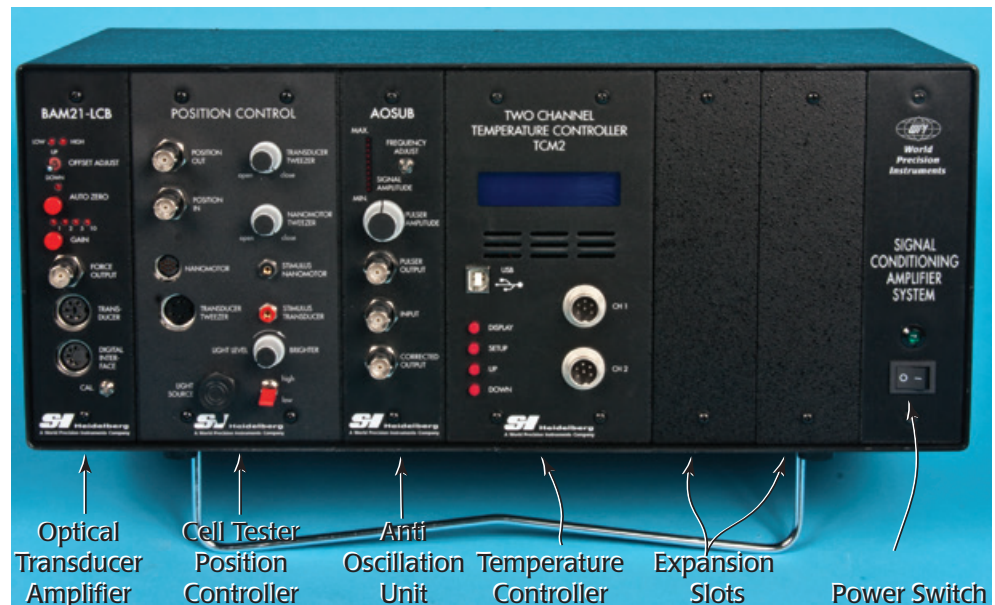
Fig. 3–The front panel of a Signal Conditioning Amplifier System configured for a Cell Tester shows the SI-BAM21-LCB, the Position Controller and the SI-AOSUB.
