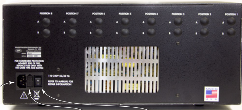
Power Connector Fuse Housing Master Power Switch
