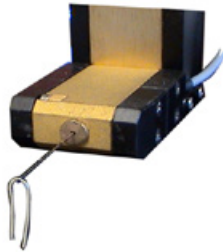
Fig. 33—Suspend a 80mg weight from the end of the force transducer.
