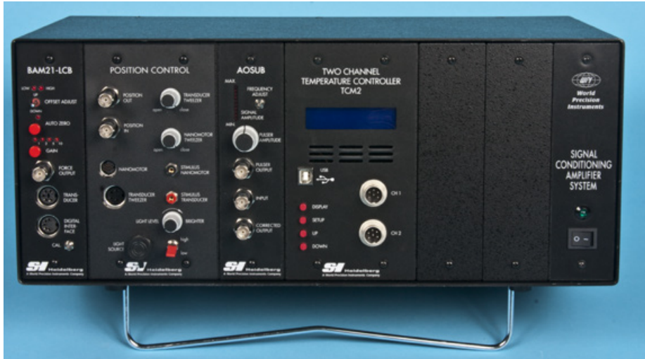
Fig. 2—The Signal Conditioning Amplifier System is a flexible chassis that is specifically configured for the SI-CTS200 (Cell Tester).
