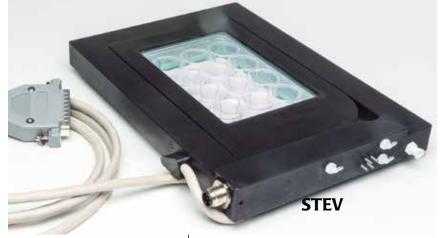
(Above) All the connection ports for the STEV are located on the same side of the unit.
