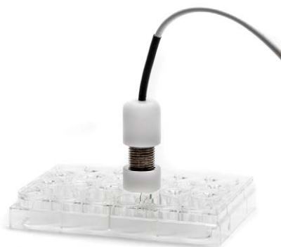
Fig. 9—The STX2-PLUS sits securely over a well insert.
