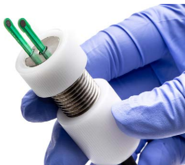
Fig. 7—The electrode length is properly adjusted.
