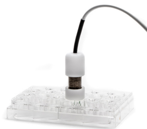
Fig. 12—The STX4 sits securely over a 24-well insert.
