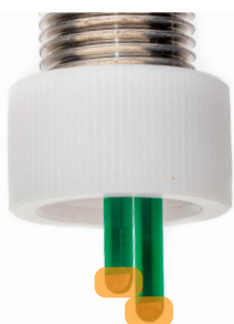
Fig. 33—Verify the electrode sensing tips (highlighted region) on both blades stay fully immersed in a conductive liquid (cell culture media or buffer) during measurement. You need to have adequate apical and basolateral volumes to get a stable reading.
