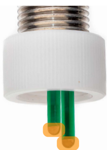
Fig. 33—Verify the electrode sensing tips (highlighted region) on both blades stay fully immersed in a conductive liquid (cell culture media or buffer) during measurement. You need to have adequate apical and basolateral volumes to get a stable reading.
