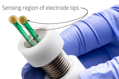
Fig. 10—The exposed electrode blade lengths are properly adjusted. The arrows highlight the coated sensing region.
