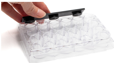
Fig. 28—Position the fixture over the filled wells of a 24-well plate.
