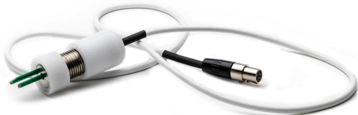
Fig. 27—The STX4 electrode is assembled and ready for use.
