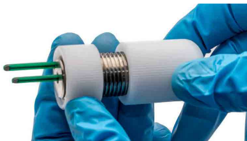
Fig. 18—Twist off the front ring to remove it.
