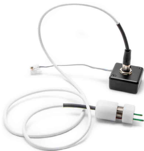
Fig. 31—Plug the STX4 into the 99675 cable to use the electrode with an EVOM2. The 99675 cable is sold separately.
