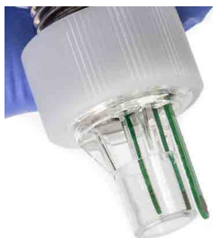
Fig. 11—The outer electrode reaches close to the bottom of the well plate, and the inner electrode does not touch the membrane.
