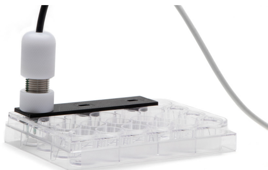
Fig. 30—The electrode is inserted so that the long blade is near the wall of the well and the short blade is near the center of the well.
