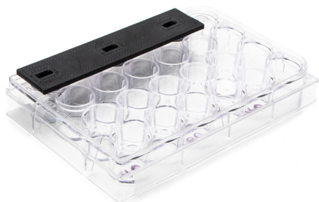
Fig. 29— The test fixture is inserted all the way inside the wells of a 24-well plate.
