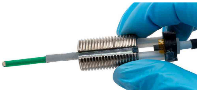
Fig. 24—Press the blade with the foam positioning padding through the center hole. The outside blade was removed so you can see the connection port.
