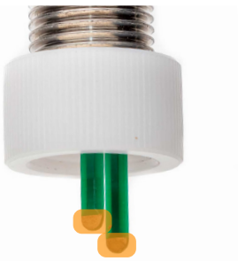
Fig. 33—Verify the electrode sensing tips (highlighted region) on both blades stay fully immersed in a conductive liquid (cell culture media or buffer) during measurement. You need to have adequate apical and basolateral volumes to get a stable reading.
