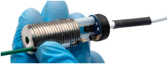
Fig. 22—Align the pins with the connection port and gently press the blade in place.
