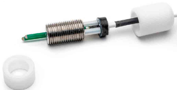
Fig. 20—Twist the back of the casing off to expose the connection ports for the blades.
