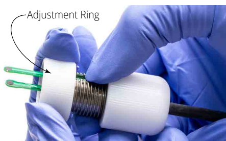
Fig. 9—Rotate the front ring to adjust the exposed length of the electrode blades.
