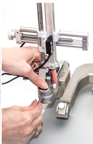
Fig. 5—(Left) Position the turret over the post and slide it into place.
