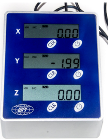
Fig. 13—(Left) The digital display is battery operated and has controls to independently power and zero all three axes.
