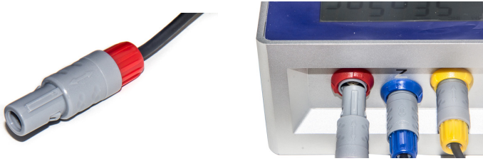
Fig. 15—(Left) Each connector has a notch that must be properly aligned with the connection port on the back of the controller.
