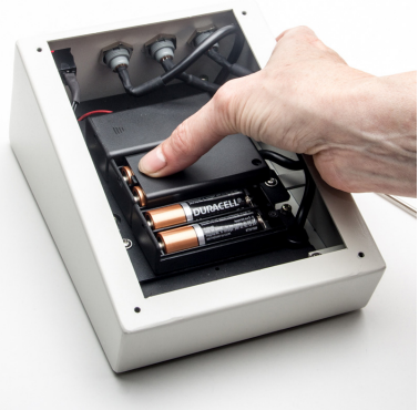
Fig. 21—(Right) Press and slide the battery covers to the right to remove them.
