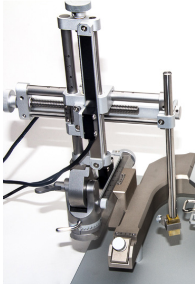
Fig. 8—(Left) Align the probe holder with the V-shaped notch on the manipulator arm.
