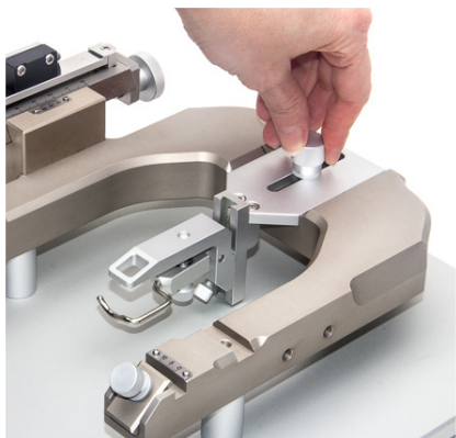
Fig. 3—(Left) Remove the thumbscrew, flip the rat adapter and reinstall the thumbscrew.
