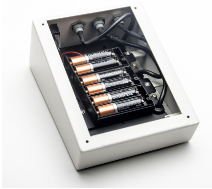
Fig. 22—The controller holds six AA batteries.
