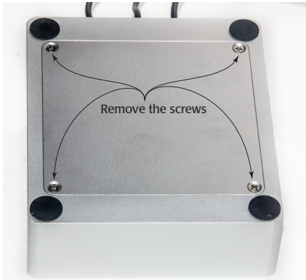
Fig. 19—First, remove the four screws on the bottom of the controller.
