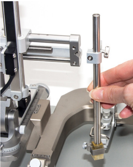
Fig. 8—(Left) Align the probe holder with the V-shaped notch on the manipulator arm.
