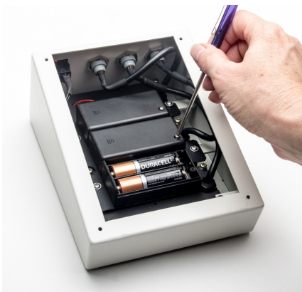
Fig. 20—(Left) Remove the screws holding the battery covers.
