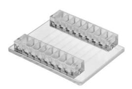
Each 10 pack contains 80 assays. These biochips are compatible with confocal microscopy. Compatible with Mirus Evo nanopump, ExiGo, UniGo and 4U microfluidic pumps for low shear stresses of 0.1–2 dyne/cm² (water-based solution) and 0.45–9 dyne/cm² (whole blood) and for high shear stresses of 20–40 dyne/cm² (water-based solution) and 90–180 dyne/cm² (whole blood). Compatible with Kima pump for cell culture.
