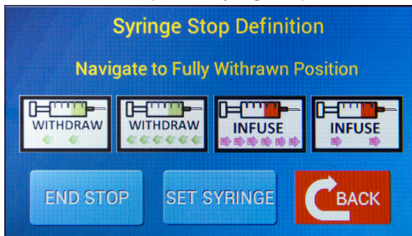
Fig. 15—The Syringe Stop Definition screen lets you define the limits of travel for the pump.
