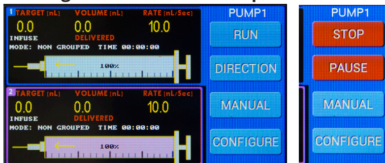
Fig. 29—Use the Command screen to control the pumps.
