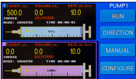
Fig. 10—Channel 1 is selected, and PUMP1 is shown with a blue background. When Channel 2 is selected the background turns pink.
