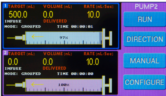
Fig. 36—Pump 2 is the Master pump, and Pump 1 is the slave in this example.
