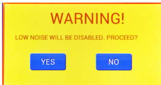
Fig. 22—Warning message appears to let you know that the motors will be re-engaged and the Low Noise Recording period will end.
