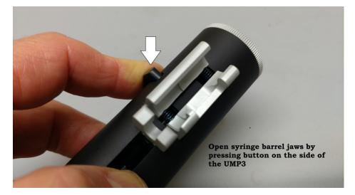
2. With the jaws held open, install the barrel of the syringe into the jaws with the flange of the syringe located between the jaws and the flange retainer. Release the button. The jaws close by spring action.
