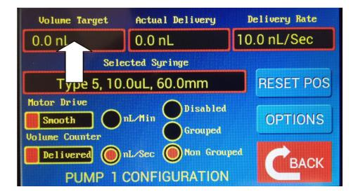
8. The "Volume Target" screen appears. Use the numerical keypad to enter the volume you wish to dispense in nanoliters. The value used in this quick start example is 1000 nL.
