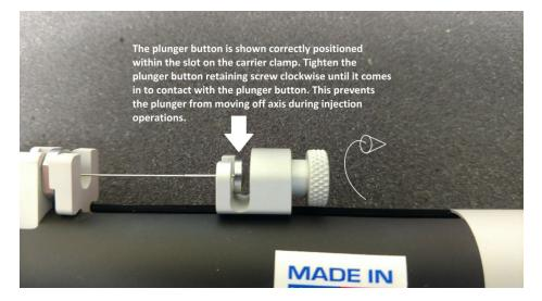
4. Center the plunger button in the carrier slot and then tighten the carrier retaining screw so that it comes into contact with the plunger button to secure it. The plunger button should be centered in the carrier slot so that the plunger shaft is parallel with the axis of the syringe body.
