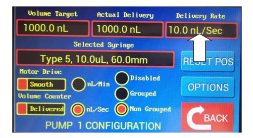
10. The "Volume Rate" screen appears. Use the numerical keypad to enter a desired injection rate in nL/sec. In this example 500 nl/sec has been entered. Touch "ENTER" to set the delivery rate and return to the "CONFIGURATION" screen.
