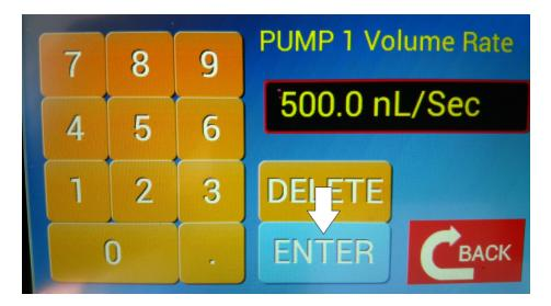
11. The configuration screen shows that a target volume of 1000 nL has been entered and a delivery rate of 500 nL/s has been entered. Touch "BACK" to return to the syringe status {Home} screen.
