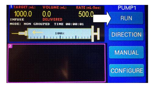
13. The injection will run until 1000 nL is injected, and will then halt automatically. Press the "STOP" button at any time to manually halt the injection before the programmed amount is dispensed. Pressing "Stop" resets the volume counter.
