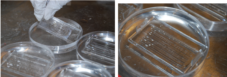
Fig. 2—(Left) The Z-Molds are placed with the ridged side down in a liquid agarose gel.
