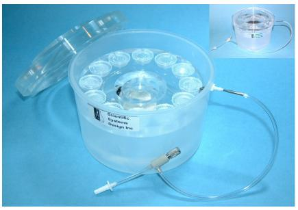
the 'C' rings. This ensures BSK12 Brain slice keeper with rings and net in place and with lid in circulation of fluid over the top place (inset). A needle valve is used to control the flow of oxygen
