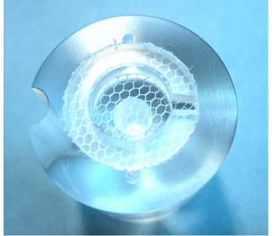
View of insert with acrylic ring wedging removable nylon net.
