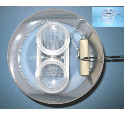
viable for many hours in these BSK5-2 viewed from above. Brain slice keeper with rings and net in place and with lid in place (inset). An included needle valve is placed into a water bath for used to control the flow of oxygen mixture to the ceramic bubbler.
