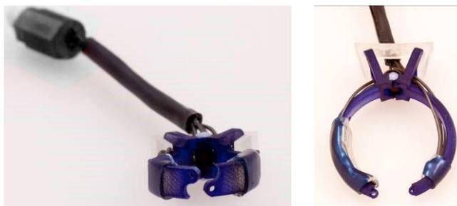
To attach the sensor using this method, first make sure that the sensor is not connected to the CME. Anesthetize the animal, then retrieve a suture needle from its packet (size 5 or finer). Although we do not recommend a specific
