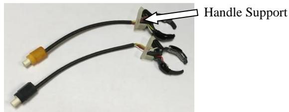
MouseOx® Plus sensors are visually differentiable from those of the original MouseOx® by virtue of the **orange** or **black** sleeve adjacent to the connector. **MouseOx® Plus sensors are not backward compatible**
