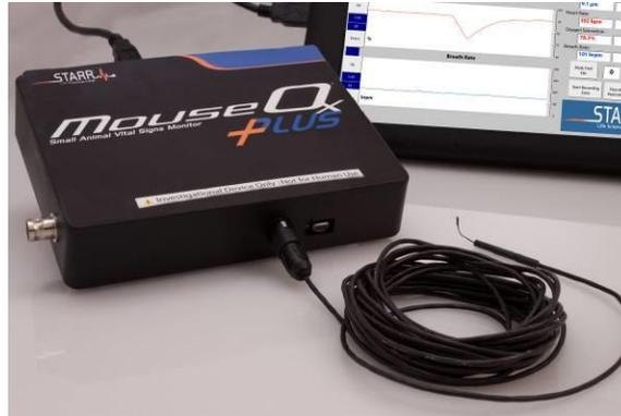
The measurement end of the probe can be used as a rectal thermometer, but can also be used in other locations. Once the sensor has been placed, you are ready to make measurements. Refer to the Software Description section below for further details.
