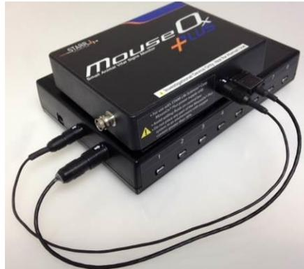
Next, connect the USB cable between the Multiplexer™ and the computer, then connect the power supply to the port on the Multiplexer™. The order of connection is inconsequential. Finally, connect the different Universal Cables into the channels of your choice.
