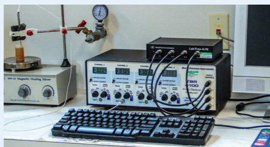
This is a typical laboratory setup of a WPI free radical analyzer with data acquisition system.
