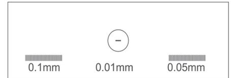
**Glass-Slide Micrometers (504606)** are placed below your petri dish for injection sample-to-target measurement.
