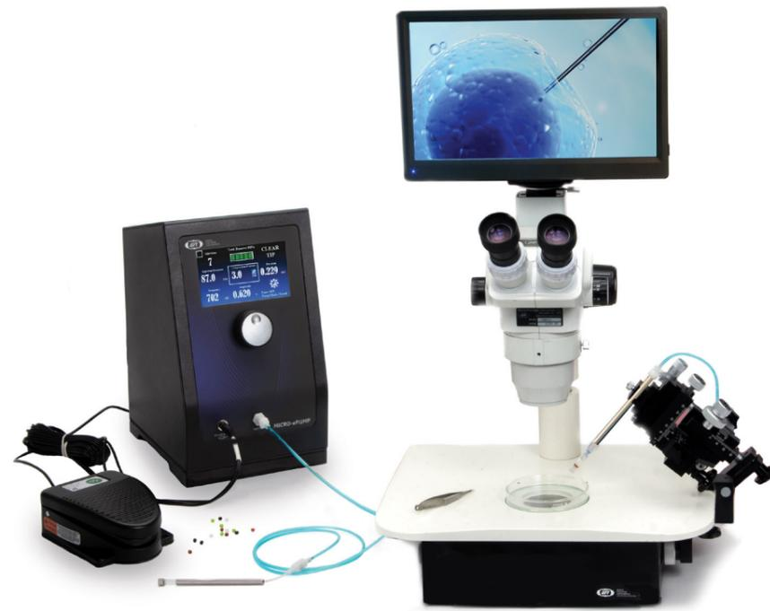
The full microinjection system presents components which optimize both visibility and application experience. Our new generation pressure microinjectors (**PV850**, **µPUMP**, and **Micro-ePUMP**) offer a streamlined solution for ultra-low volume delivery for cell transfection.
